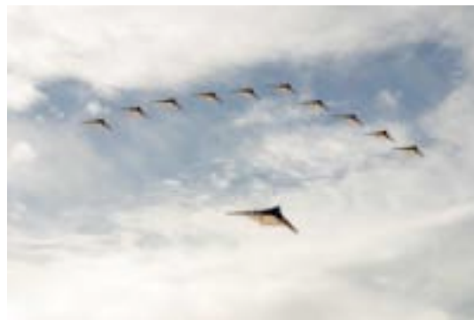
Figure 21. "Artist's" concept of formation flight for low cost cargo transportation. Use of configurations especially tailored for formation flight can amplify potential savings.
