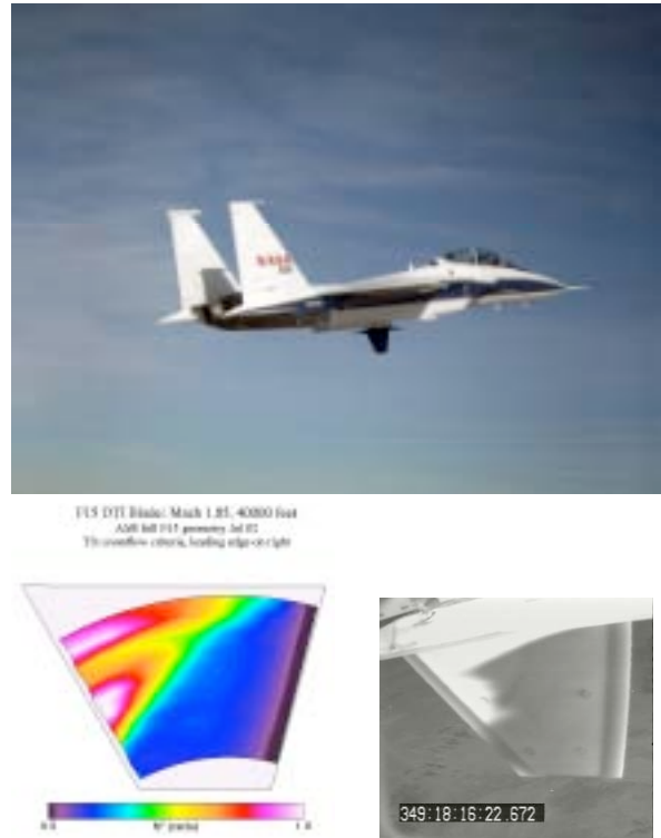
Figure 4. Computed amplification factors on supersonic test wing (left). Infrared image of test wing showing turbulent areas in white (right). F-15B with test wing mounted below (top).
