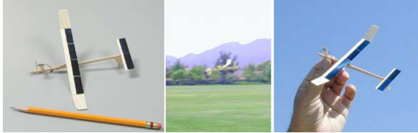
Figure 14. Matt Keenon's 1.7g solar-powered aircraft.
