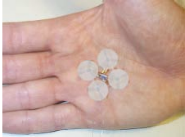
Figure 12. Mesicopter studies included optimal rotor design and testing of very small vehicles, including constrained tests of this 4-rotor design.
