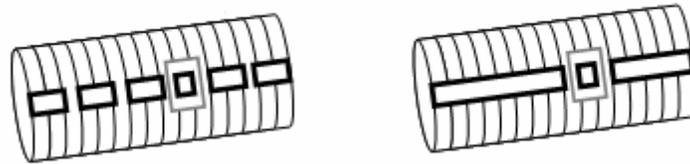
Figure 14.3: Left: conventional, discrete windows. Right: Stretched windows.
