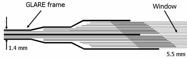
Figure 14.6: Cross-section at the edge of window panel
