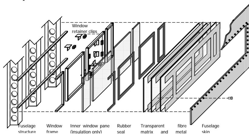
Figure 14.5: Schematic representation of the laminated window panel buildup
