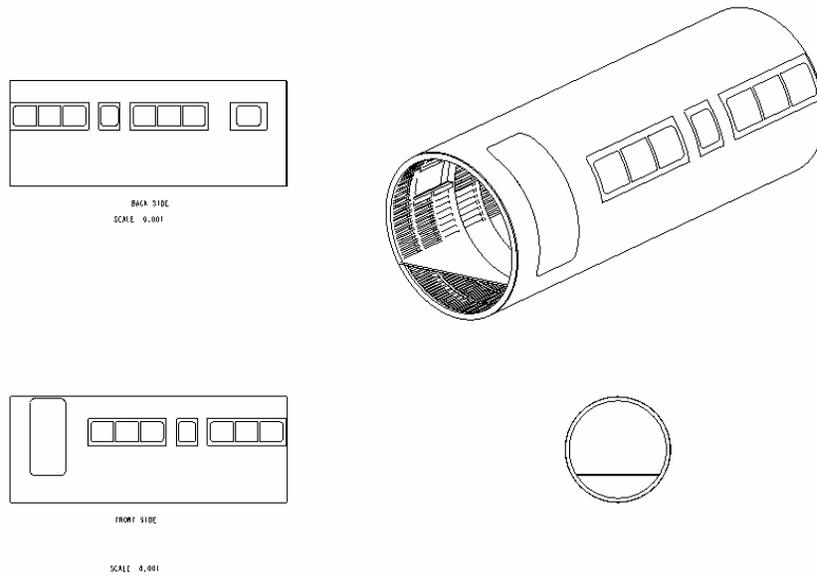
Figure 14.7: Technical drawings of the fuselage with enlarged windows
