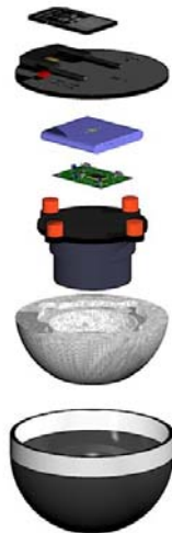
Figure 9: Exploded view of the imaging subsystem
