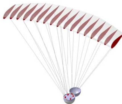
Figure 11: CATIA 3D model of the kite and capsule
