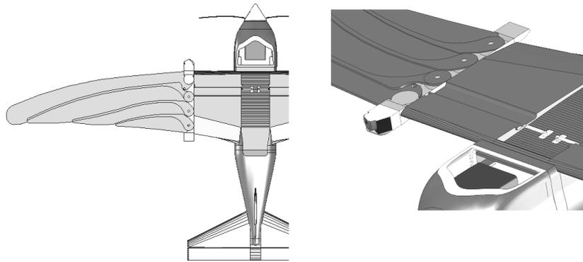
Figure 15.3: Top view and detailed view of the multiple joint feather-like morphing wings.
