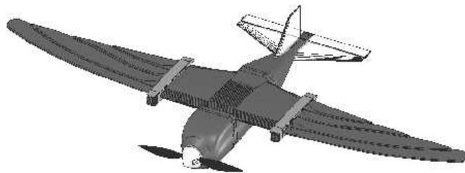
Figure 15.7: The final design concept of RoboSwift
