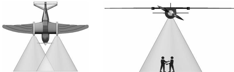
Figure 15.4: The wing-mounted cameras and the belly camera combined with the propeller in the nose (top view and front view respectively).
