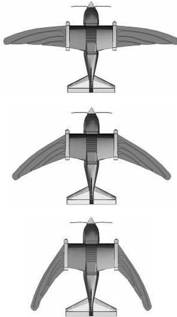
Figure 15.8: Top view of the sweeping of the morphing wing for 5°, 25° and 50° sweep
