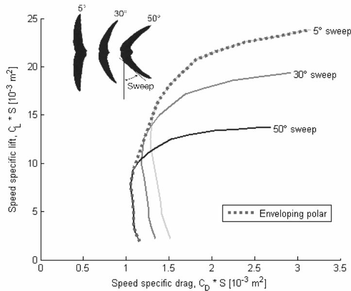
Figure 15.5: The lift drag polar of RoboSwift showing the extended flight envelope due to morphing.
