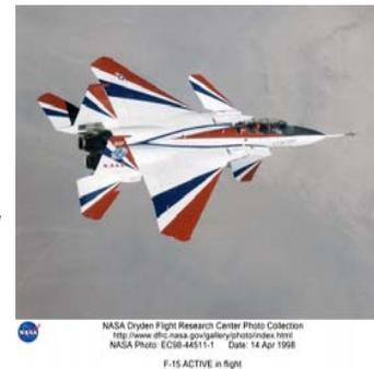
*NASA's F-15 Research Aircraft can be flown with varying nozzle positions to generate a variety of validation data*
