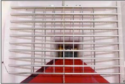
*Improved Icing Research Tunnel to enable research on super-cooled liquid droplets.*
