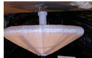
*The IRVE flight test vehicle is shown at left during a ground deployment test*
