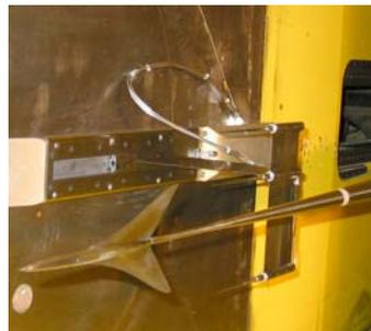
*Conventional wind tunnel mounting techniques distort the aft end of the model being tested.*
