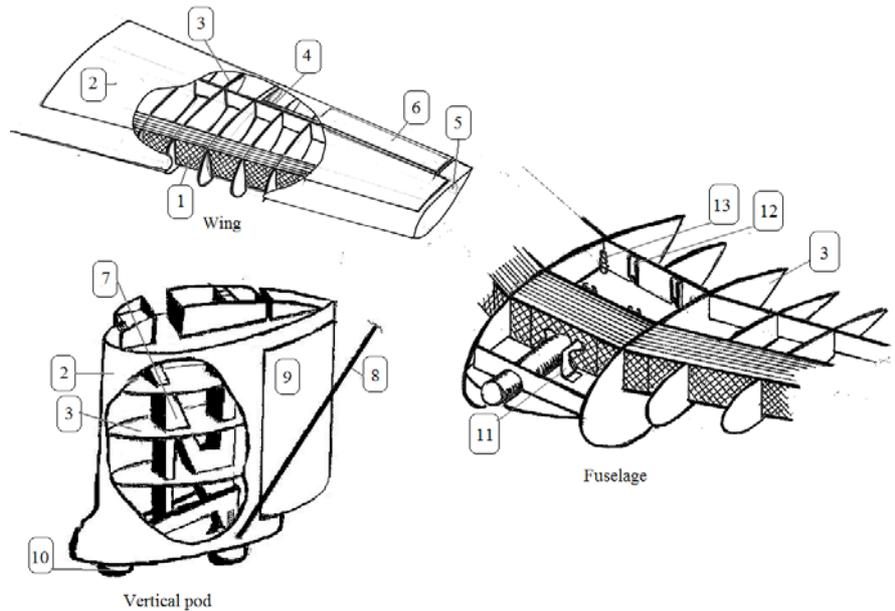
Figure 6.6: The aircraft's structure
