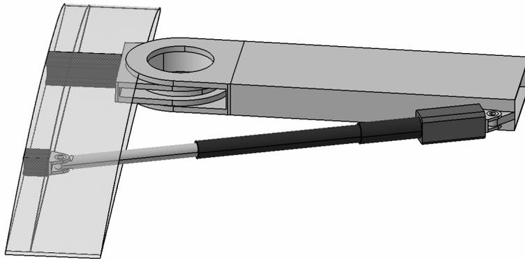
Figure 13.3: Swing wing mechanism
